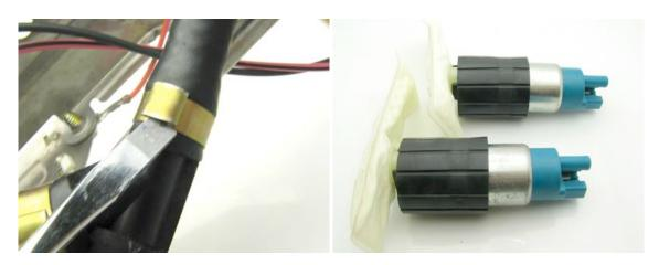
3 – reuse the pump isolators and install the fuel sock and sock retainer
